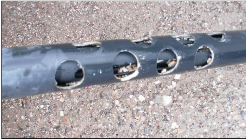
Figure 31. Gravel and sand deposited in the Hydrolab housing and sensor guard by high flows in Almo Creek.
