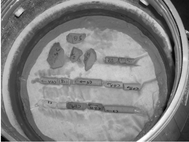
Figure 7. Rock cores and solid rock slabs in the water retention tank, in which the water level can be varied (Hendrickx's soil physics laboratory at New Mexico Tech)
