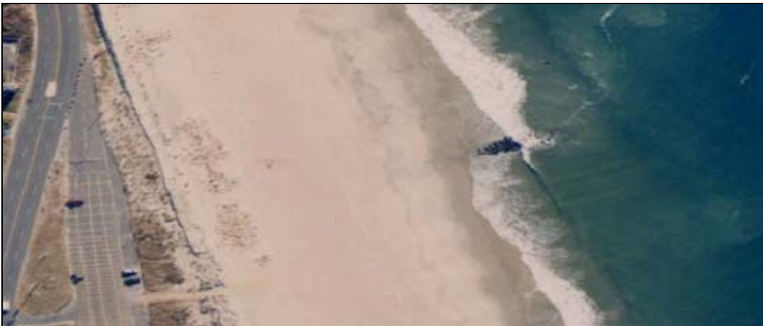
Figure S5.8. This aerial view of GATE-SHU demonstrates the offset of the shoreline at an interruption. Source: NPS-GATE
