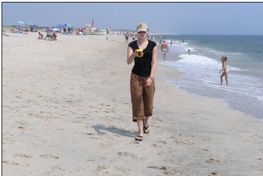
Figure S5.7. Conducting the survey and holding the GPS receiver. The operator walks along the wet/dry line on the beach face to capture the position of the neap high-tide swash line.
