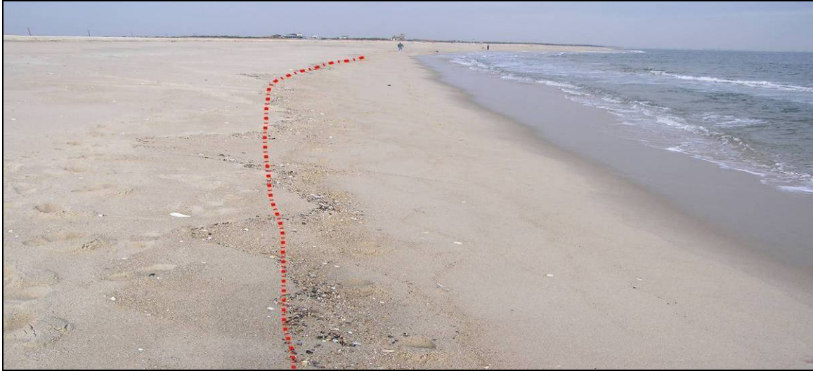
Figure S5.6. The high-tide swash line (red dashed line) has small irregularities that will be smoothed, recording the average position of the line.
