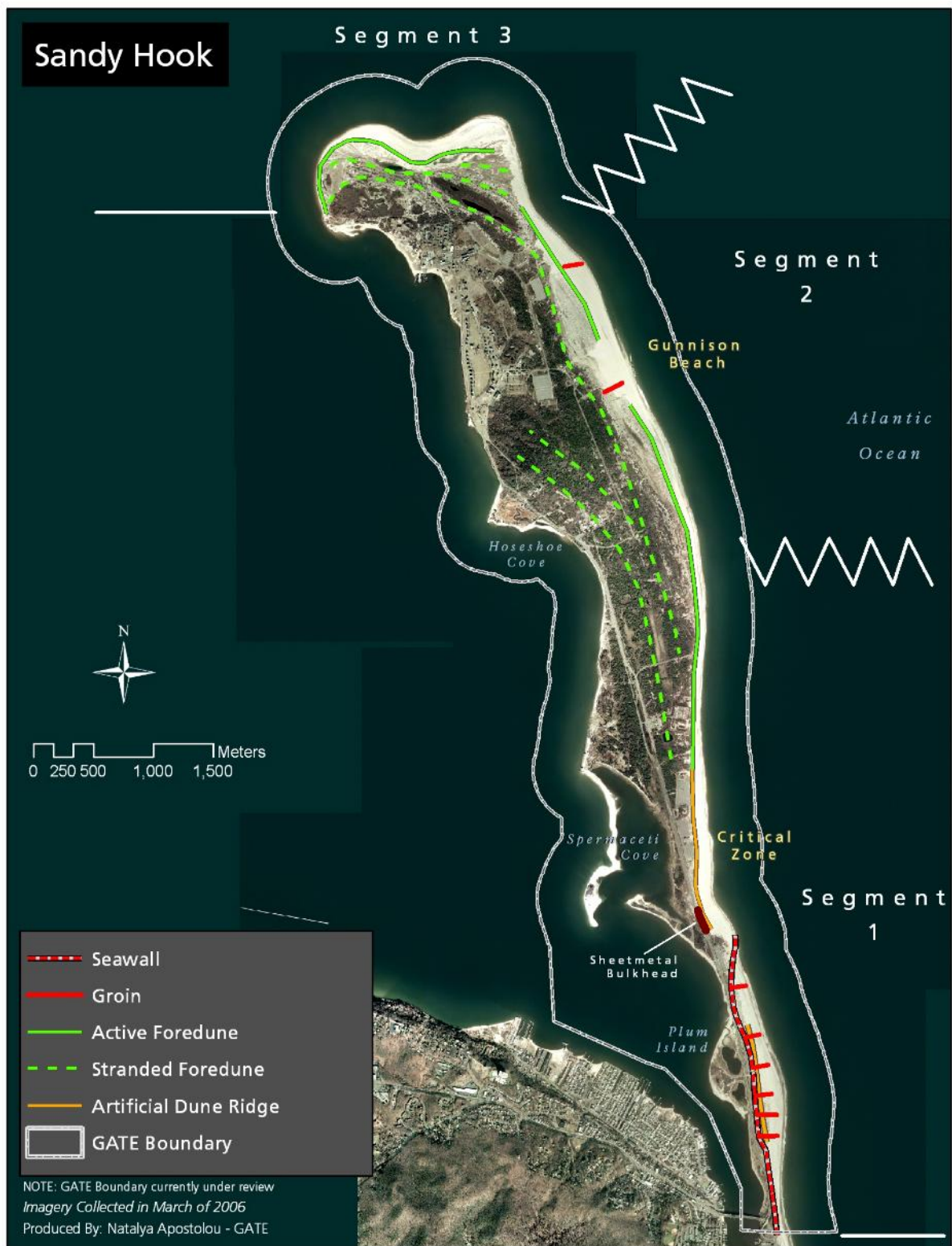
Figure 8. Coastal topography and engineering structures on the Sandy Hook Unit. The natural dune-beach system is divided into the active units and those which have been stranded inland as the spit has evolved.
