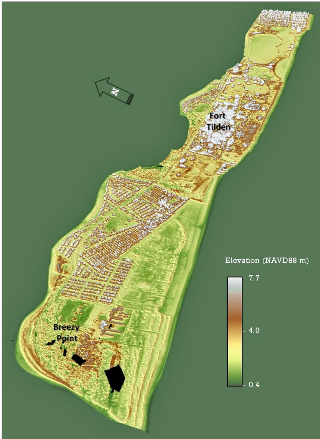
Figure 21. Coastal topography of Breezy Point spit, derived from first-return measurements collected in 2005 using the NASA Experimental Advanced Airborne Research LiDAR (EAARL); part of a collaborative effort among the USGS, NASA, and NPS. This data set provides metrics of the topographical elements of this site.
