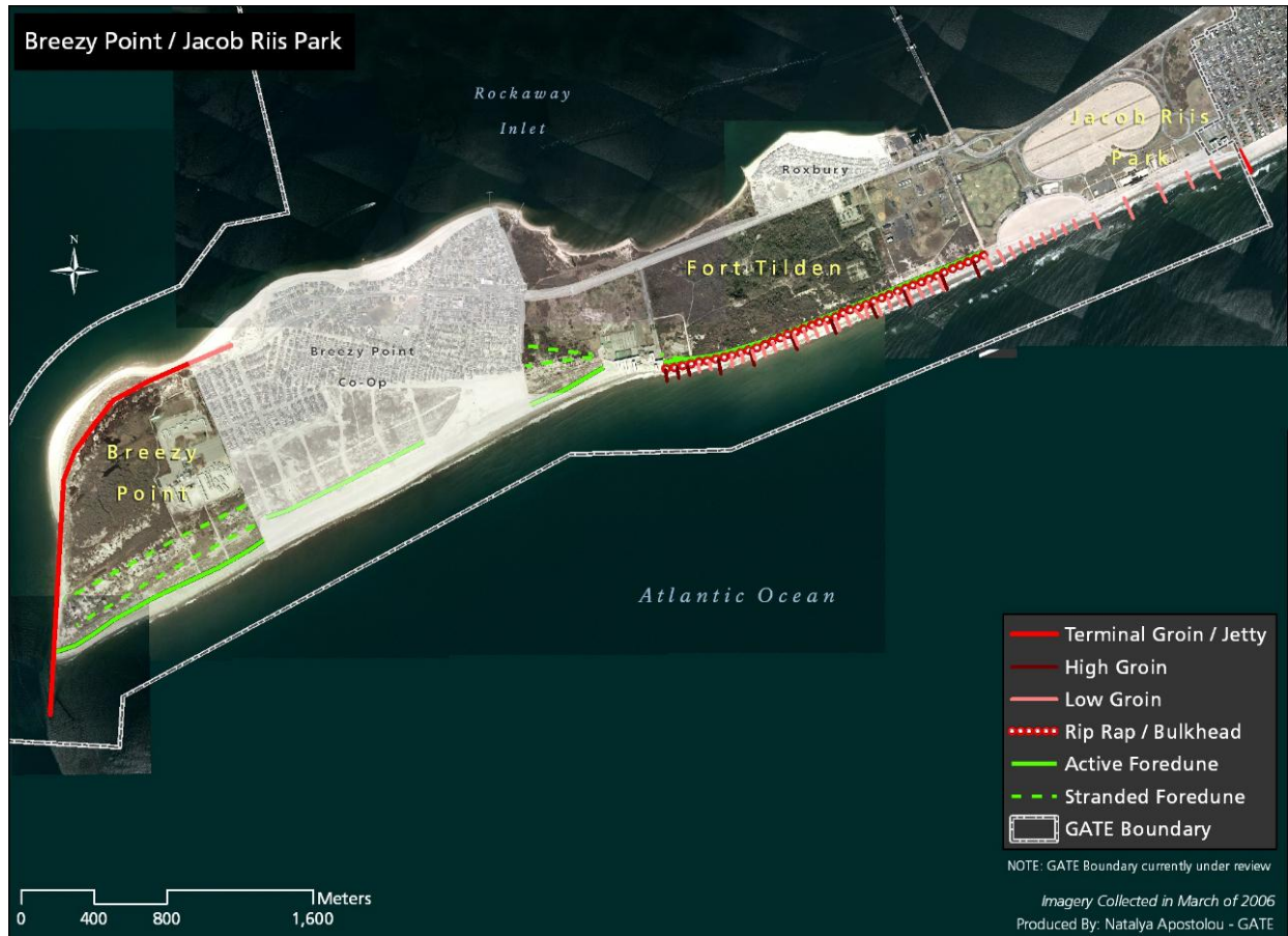
Figure 19. Ocean coast extends from the jettied Rockaway Inlet updrift to the eastern margin of Riis Park. The offset at the western portion of Fort Tilden follows the trend of the shoreline before construction of the Breezy Point jetty in 1933.
