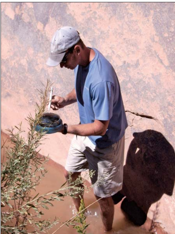
Photo 2-3. Measuring solar radiation with a Solar Pathfinder™ at Coyote Gulch, Glen Canyon National Recreation Area.
