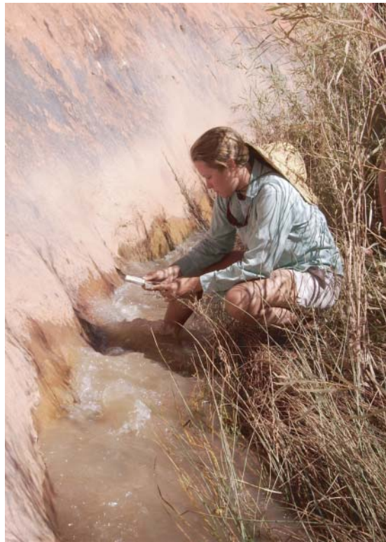
Using a densiometer to estimate riparian canopy cover at Coyote Gulch, Glen Canyon National Recreation Area.
