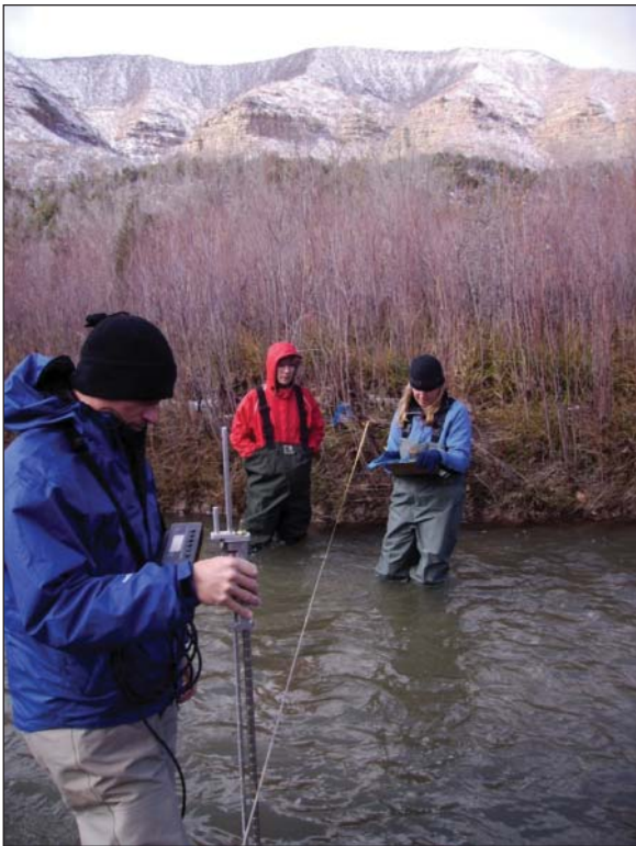
Photo 2-1. Measuring flow velocity in the Mancos River, Mesa Verde National Park.
