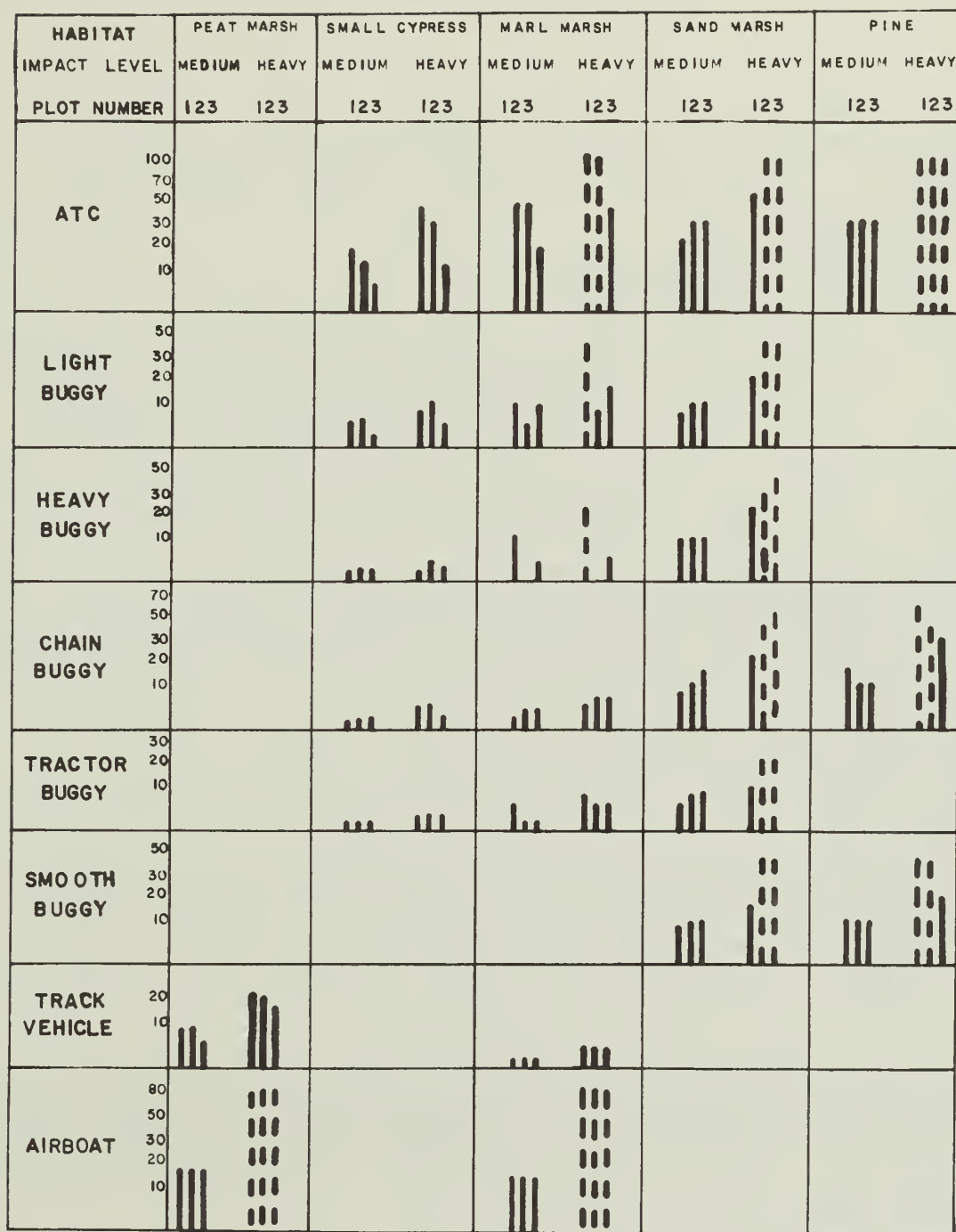
Figure 9. Relative numbers of passes required to produce medium and heavy impacts in three test plots in each habitat. A dashed line indicates the vehicle could not produce a heavy impact in that number of passes.
