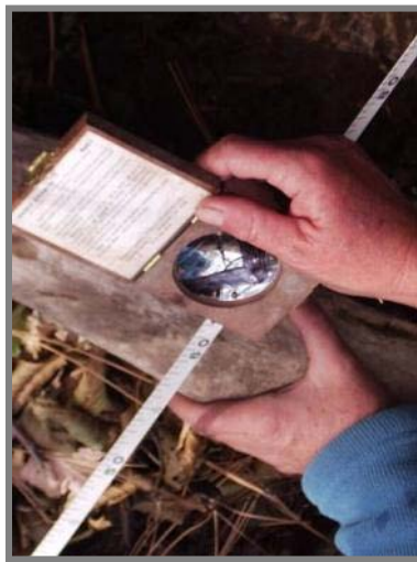
Figure S.23.2. Using a spherical densiometer to measure riparian canopy closure.
