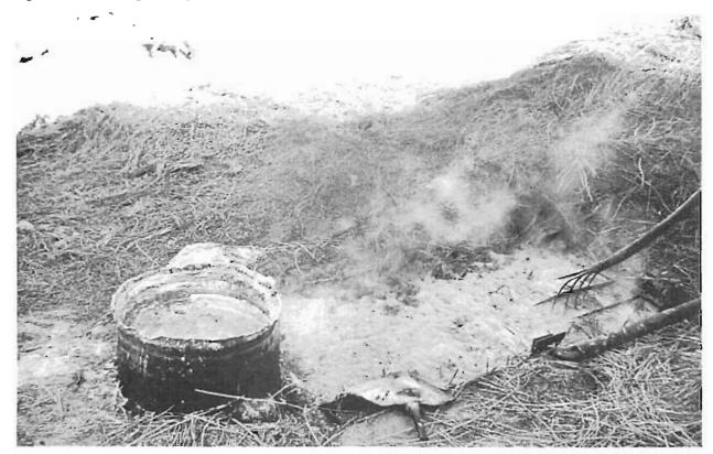
Fig. 27. Waxey foam on top of a boiling vat with steel drum mold to the left. The manufactured pitchfork is rare. Mariscal Canyon.
