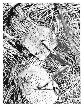
Fig. 29. Two well-used skimmers handmade from tin cans.
