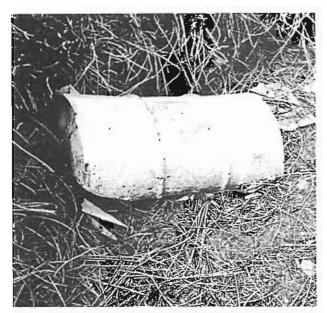
Fig. 36. Block of cerote from a half-barrel mold. Lower Canyons.
