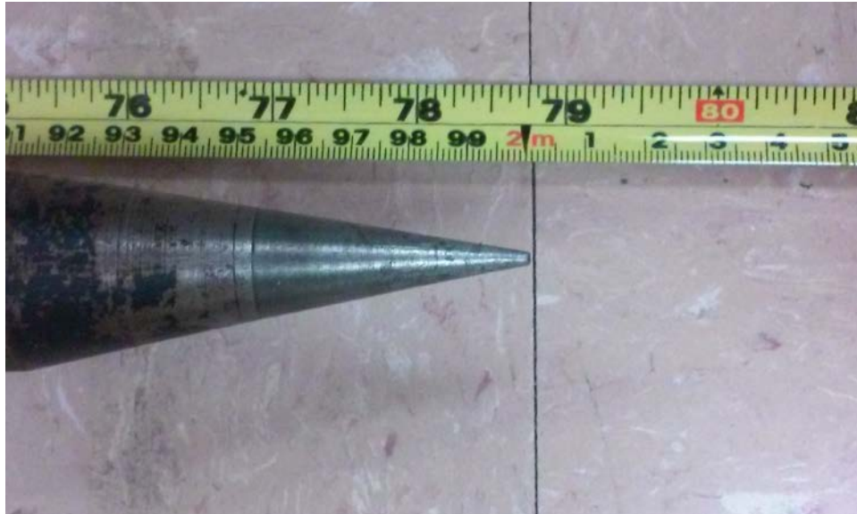
Figure 6.6. Verifying the length of the central leg of a fixed height GPS tripod.
