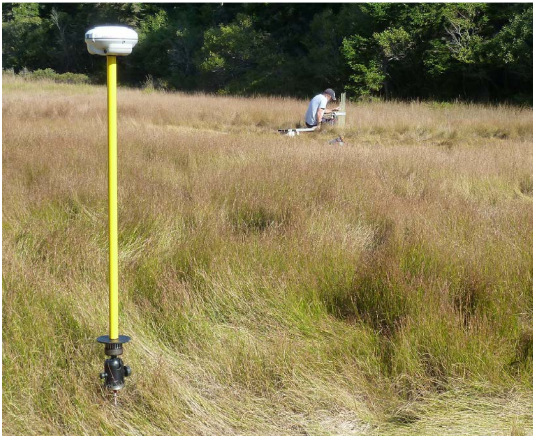
Figure 6.3. Foreground: a static GPS occupation of a SET mark (the Local Control Mark) using a custom GPS antenna adapter; in the background is another, nearby SET sample station being measured (Acadia National Park, ME, USA).
