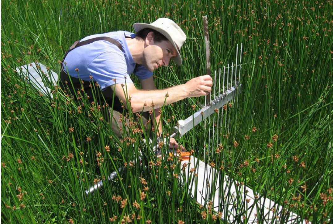
Figure 4.20. Reading pin heights (Eastern Neck NWR, MD, USA).
