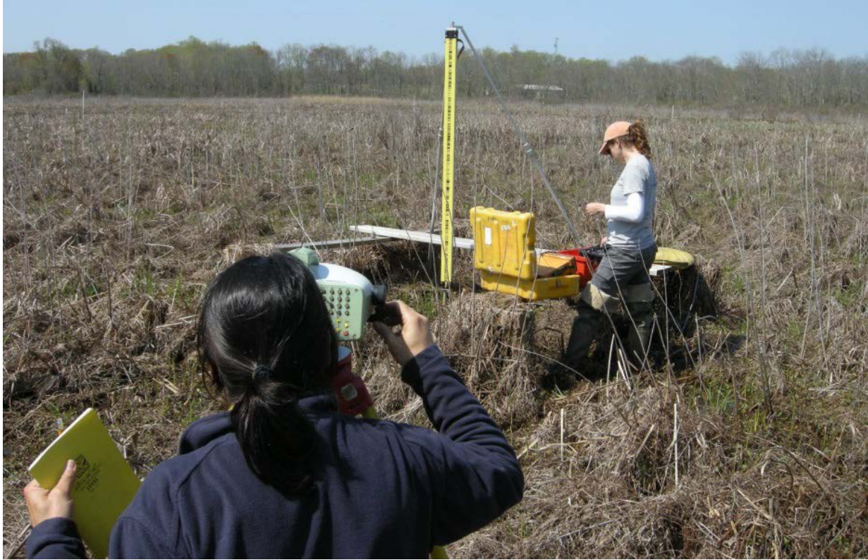
Figure 26. Digital barcode leveling is used to transfer elevations from a SET mark to other vertical infrastructure (Jug Bay, MD USA).
