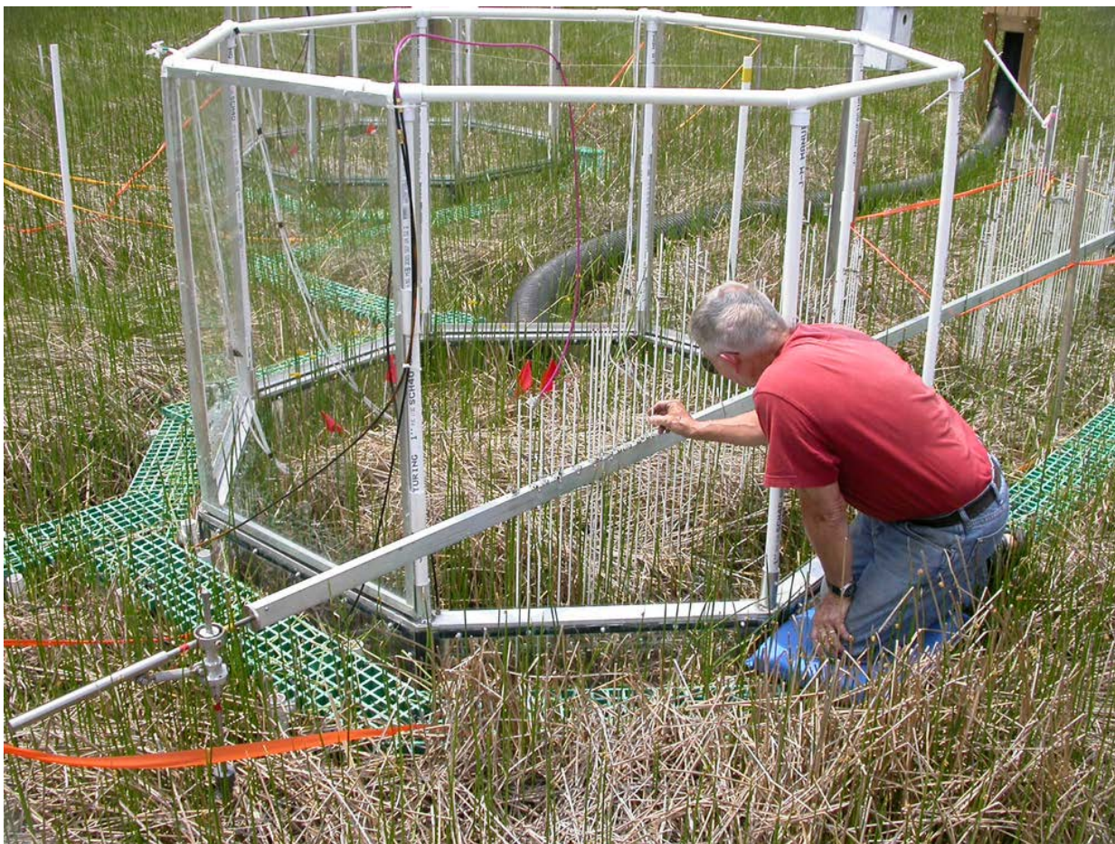
Figure 4.2. Monster Arm SET (Smithsonian Environmental Research Center, Edgewater, MD USA).
