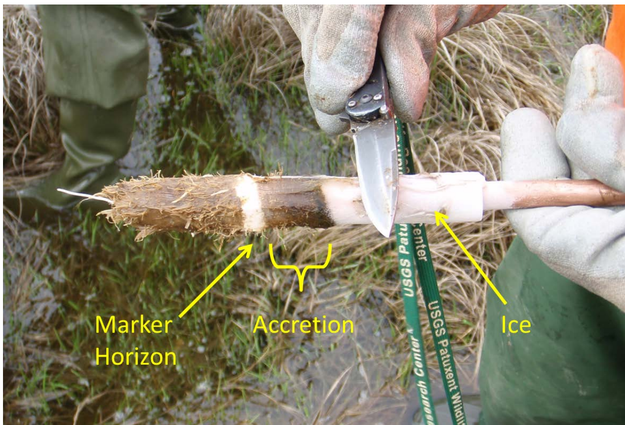
Figure 5.35. Scraping a frozen core. Marsh was covered in water which froze during coring (Gateway NRA, New York, NY USA).
