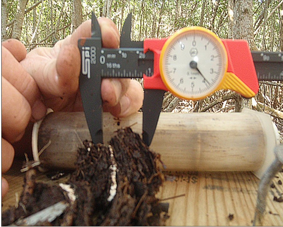
Figure 5. Example showing measurement of the accretion layer above a feldspar layer.
